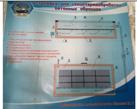
Campus 1. Heliocamera for solar energy accumulation
