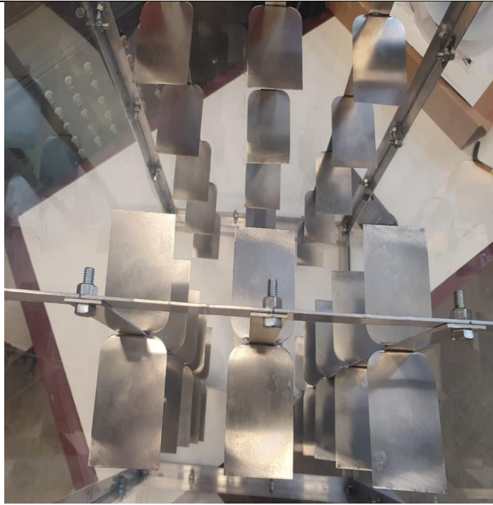
Installation program for converting the kinetic energy of the air stream into electrical energy.
